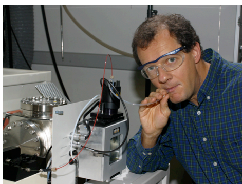
Fig. 2 A practical example of in vivo breath analysis using EESI-MS.
